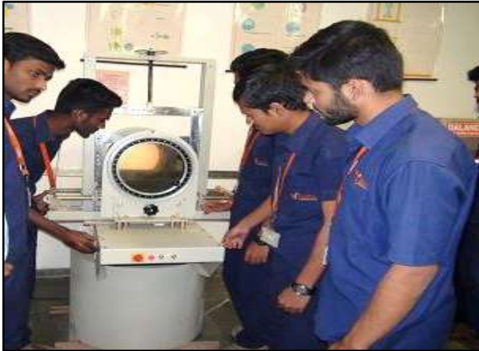
Photoelastic apparatus in Design Lab for Experimental Stress Analysis
