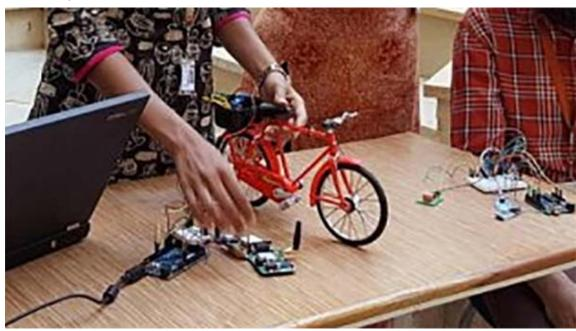
The former sensor detects the alcohol level by analysing the rider's breath while the latter detects skin contact to check if the rider has actually worn the helmet. This data is then transferred to the vehicle via a bluetooth module that either gives the green or red signal to the vehicle's ignition system.
