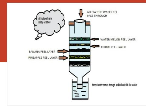
This project explores the use of protonated or activated biotic layers / semi-permeable membrane made from fruit peels waste (FPW) to reduce toxic froth from urban lakes in Bengaluru. The main pollutants are fluorides, nitrates and effluents of phosphorous released with the untreated sewage water from the industries and domestic buildings surrounding the water bodies.
