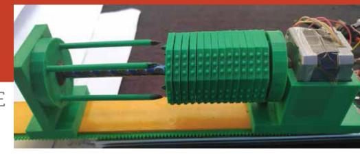
Braille Pad is a device which displays the text information using the symbols of the Braille. In the modern era of digital communication, it is important for a person to be able to access this facility and make use of it. Visually impaired have been left behind in this revolution.
