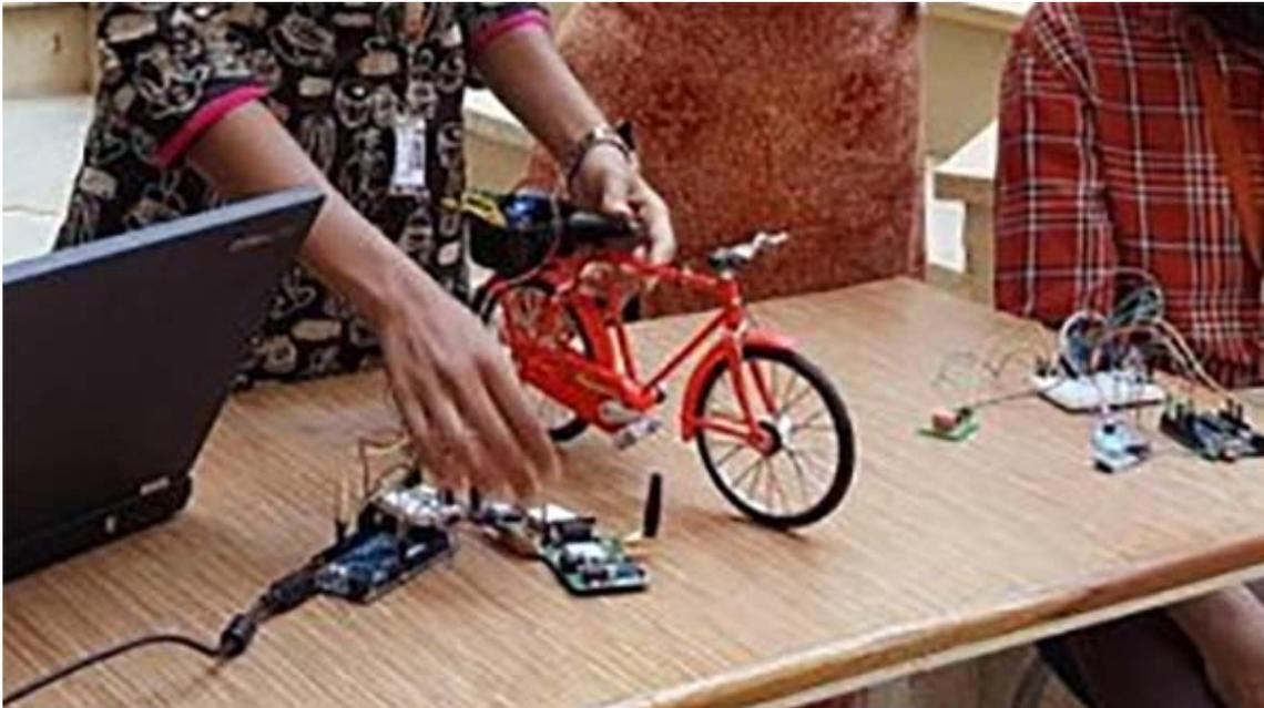
The former sensor detects the alcohol level by analysing the rider's breath while the latter detects skin contact to check if the rider has actually worn the helmet. This data is then transferred to the vehicle via a bluetooth module that either gives the green or red signal to the vehicle's ignition system.
