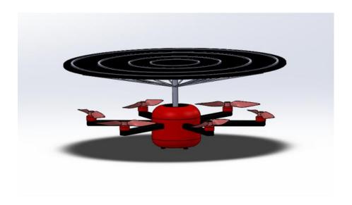
The conceptual design of the UAV for Martian Exploration by Team Abhimanyu 7.0 was a fixed wing UAV with innovative hexacopter design. The designed UAV had solar panel installed with the help of umbrella mechanism which can be stowed inside main hub during flying conditions. The UAV was designed to have maximum of 10 hops in a Martian day from sunrise to sunset.
